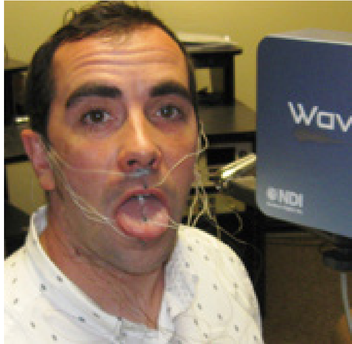
Figure 4: Sensor placement on a human subject
